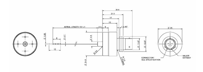
Description Thermocouple Transmitter
